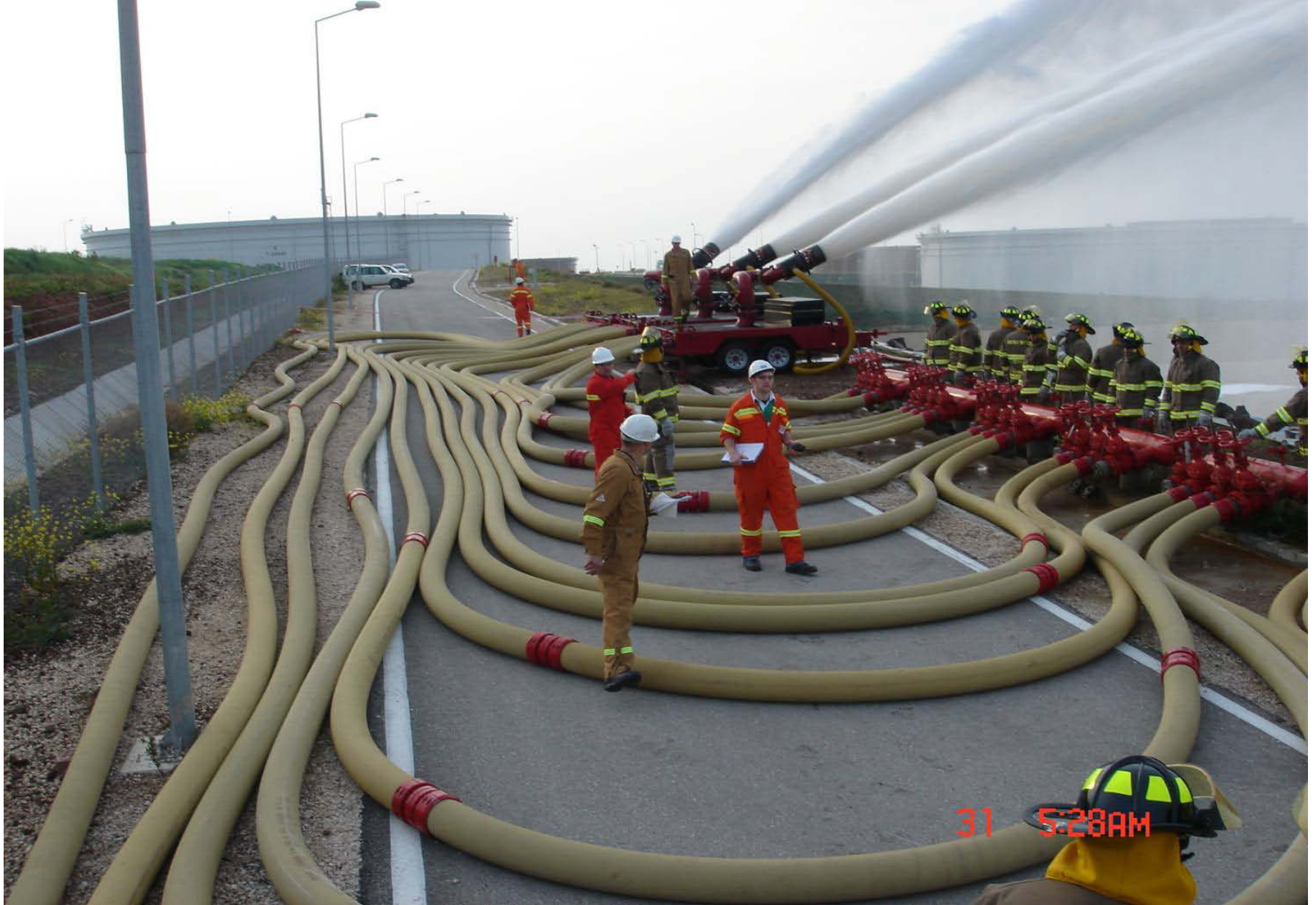
This picture illustrates on a large scale industrial water needs to control tanks of Flammable liquids to prevent BLEVE, collapse and exposures.
